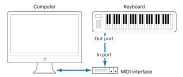
• For keyboards with tone generators: You should also connect the MIDI Out port of the MIDI interface to the keyboard MIDI In port. If your MIDI interface offers more than one MIDI output, connect any other tone generators (or other MIDI devices, such as control surfaces that require bidirectional MIDI communication) to these.
