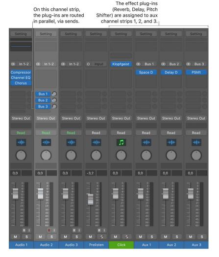
The channel strip signal is split and routed to three separate effects, one on each aux channel strip. These three independent signals are then sent back from the respective aux channel strips and combined into an output stream from the original channel strip. You can create up to eight sends on each audio, instrument, or aux channel strip.
