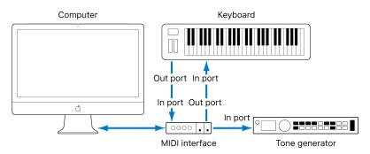
• If your MIDI interface has only one MIDI output: You need to connect the MIDI In of the second tone generator to the keyboard MIDI Thru port. A third device can be connected to the MIDI Thru of the second unit, and so on.
