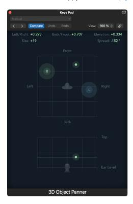
The output signal (post-fader) and panning automation data of the 3D Object Panner go directly to the Dolby Atmos plug-in for spatial processing, bypassing any other plug-ins inserted before it on the surround master channel strip.
