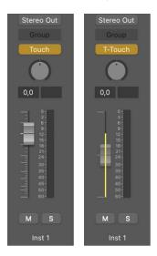
Now when you move the Volume fader during playback, it does not write completely new volume automation data but adjusts it proportionally to the existing data.
