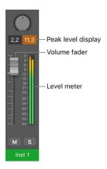
In the figure, 11.3 dB is shown in the peak level display when the Volume fader is set to 2.2 dB.
