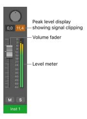
Signal clipping occurs when a signal that is too loud is fed through the output channel strip, thereby exceeding the limit of what can be accurately reproduced, resulting in distorted sound. The value shown in the peak level display lights red (on output channel strips) or orange (on other channel strip types) when the signal clips. This part of the peak level display is called the *clipping indicator*.
